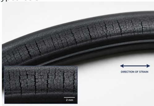
Figure 1: Failed industrial rubber part. Note cracking propagation relative to applied strain. Image generated for illustrative purposes.
