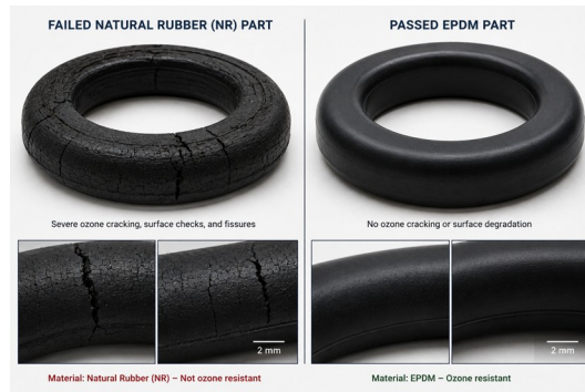
Figure 5: Comparison of Failed Natural Rubber Part with EPDM Part.
