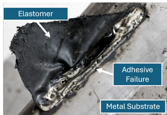
Figure 1: Magnified image generated for educational reasons showing an elastomer debonding from a metal substrate.
